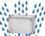
protected against water sprayed from all directions - limited ingress permitted              | 08                                               |
