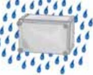
protected against direct sprays of water up to 15° from the vertical                          | 06                                               |
