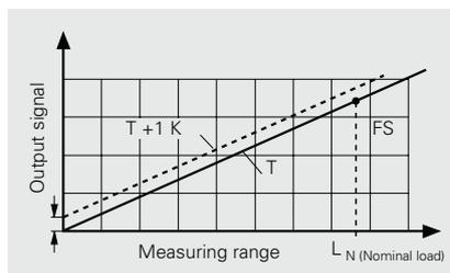
The maximum temperature coefficient (TC) of the zero signal is the largest variation of the zero signal which occurs during a change in temperature by 1 Kelvin. It is expressed in percent of full-scale per Kelvin.
