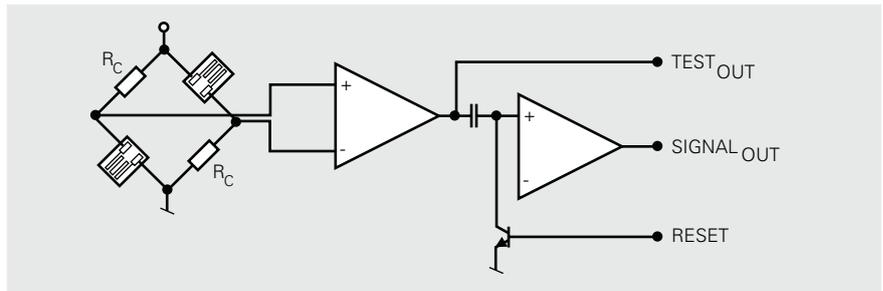
The non-tared signal is available at the output Test<sub>OUT</sub>. To prevent saturation of subsequent stages, Test<sub>OUT</sub> should ideally read between -2 V and +2 V when the sensor is installed and no load is applied. During operation this value may then be between -5 V and +5 V. The Test<sub>OUT</sub> output can furthermore be used to check the measuring chain. In case of an open bridge circuit, Test<sub>OUT</sub> goes into saturation.
